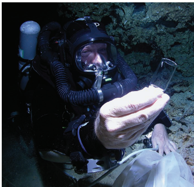
FIGURE 1. A diver uses a Megalodon closed-circuit rebreather with full face mask to collect a small shrimp, Typhlatya sp., from a cave in Yucatan. Rebreathers recycle expired gas so that no bubbles are produced.
