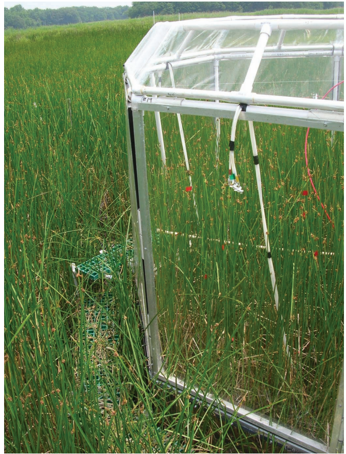
FIGURE 5. Photograph showing a chamber with a frustum that was added to all chambers before the 2007 growing season. The tubing leading to one set of porewater wells, the gas sampling tube, and the catwalk is also visible. (Photograph courtesy J. A. Langley.)
