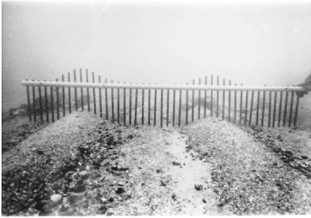
Figure 2. Sediment profile gauge in use at Stravanan Bay (Site 2) one week after storms in February 1997. The coarse surface layer of maerl gravel is thrown into megaripples 11 cm high ( \lambda=1.2 m) overlying a relatively stable layer of sediment with a higher proportion of sand and fines.
